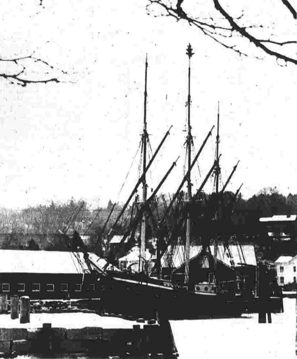
Cock-billed yards, the method of tilting wooden spars on a sailing ship during winter to prevent rain and snow from entering cracks in the wood and freezing, is a technique which can be observed at the Mystic Seaport Museum. The ship, Joseph Conrad, a former training ship for the Danish Merchant marine, is one of the many ships and nautical displays at the museum throughout the year.
